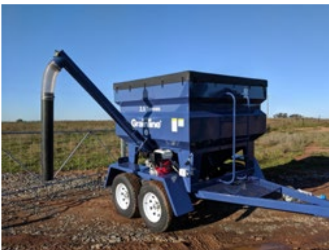
2.5 Tonne (30 bag) Feed Out Trailer including 3m x 5" Auger
